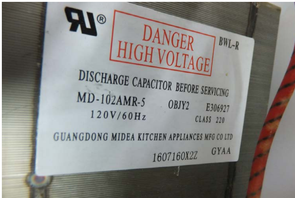
High-voltage Transformer view
