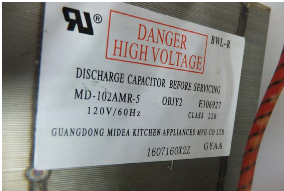
High-voltage Transformer view
