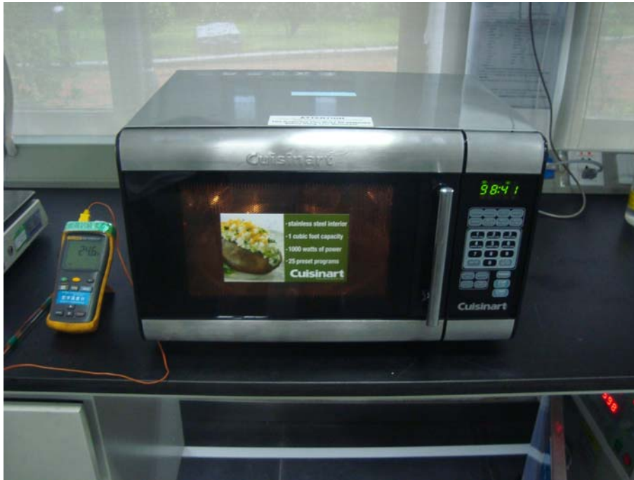
RF Output Power Test Set-Up
