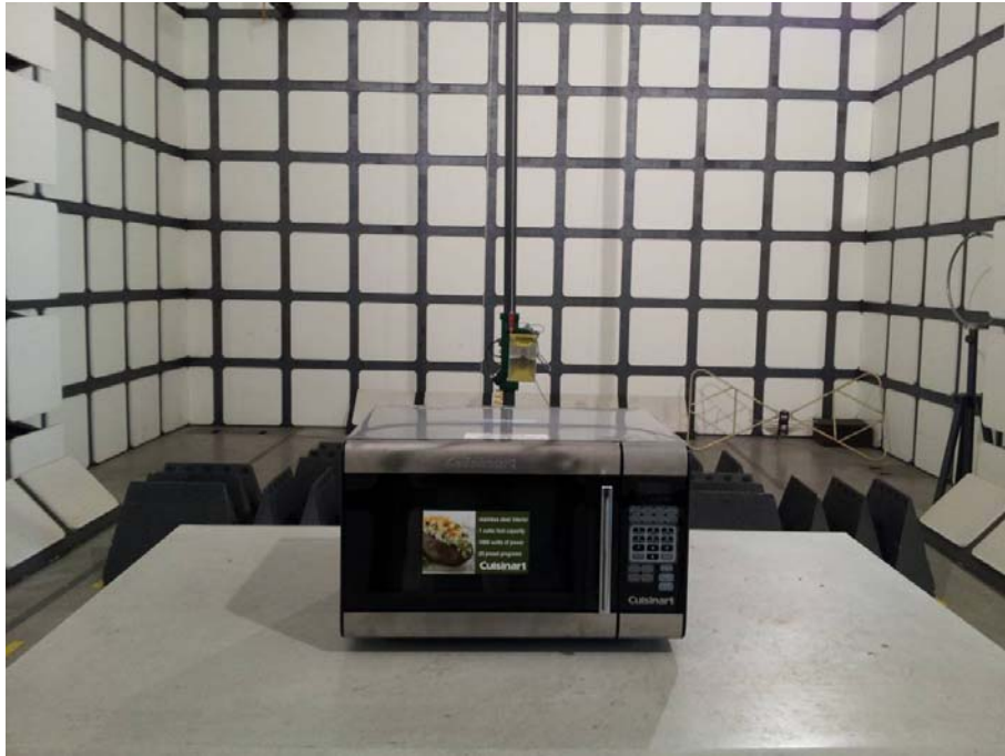
Operating Frequency Test Set-up
