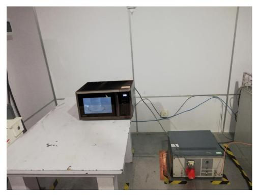
Radiated Emission Test Set-up (30 -1,000MHz):
