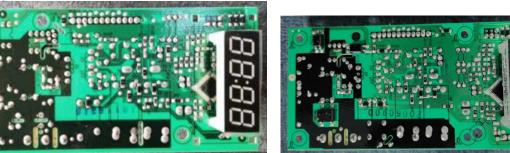
Note : New mother boad is the same of circuit function with original. They have the same input/output rating and power are identical to the original. Only some electronic components and PCB layout differences.
