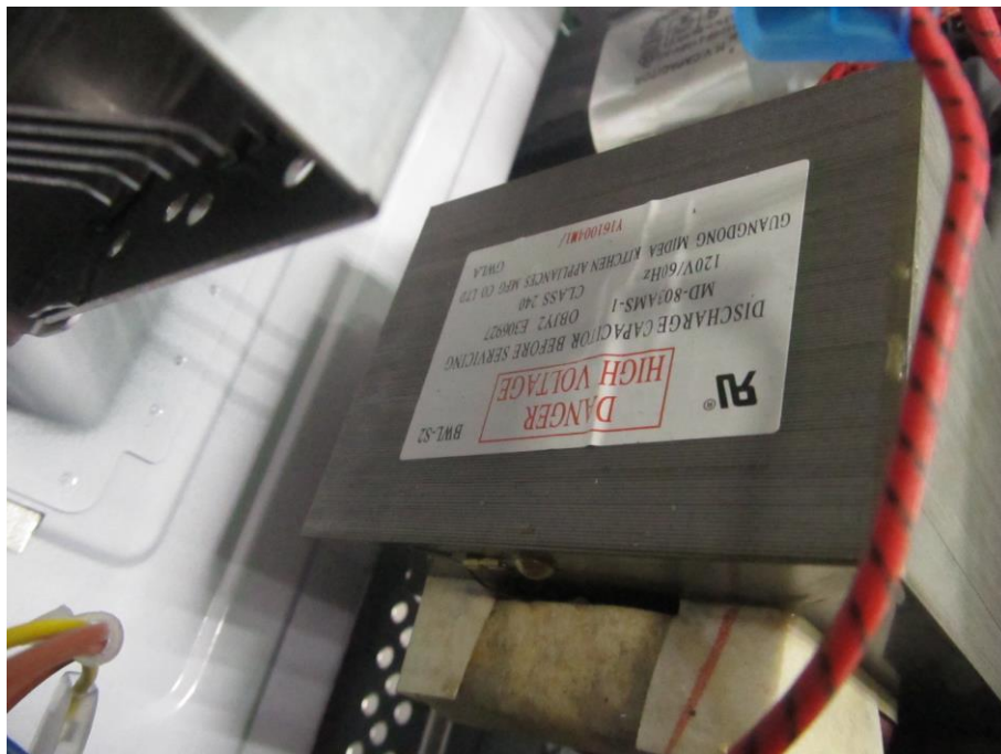
High-voltage Transformer View
