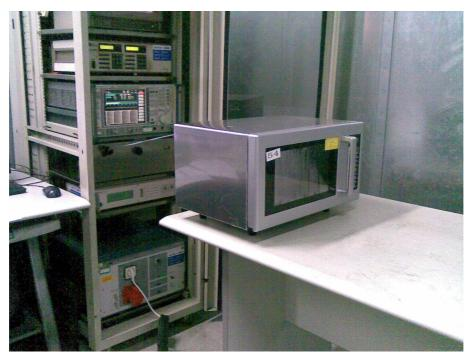
Set-up for radiation emission measurement below 1GHz
