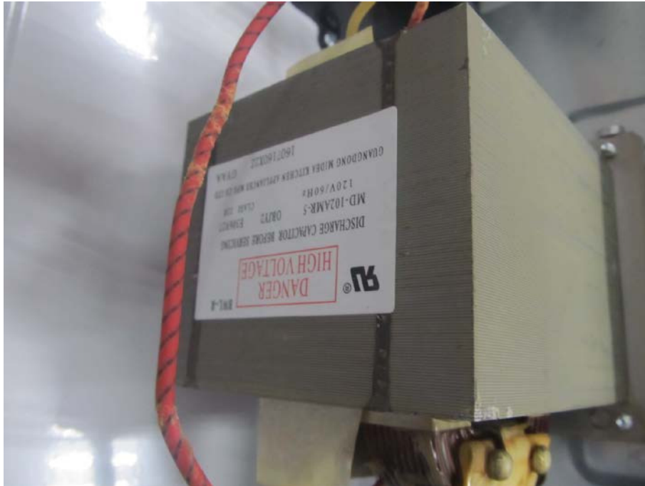
High-voltage Transformer view
