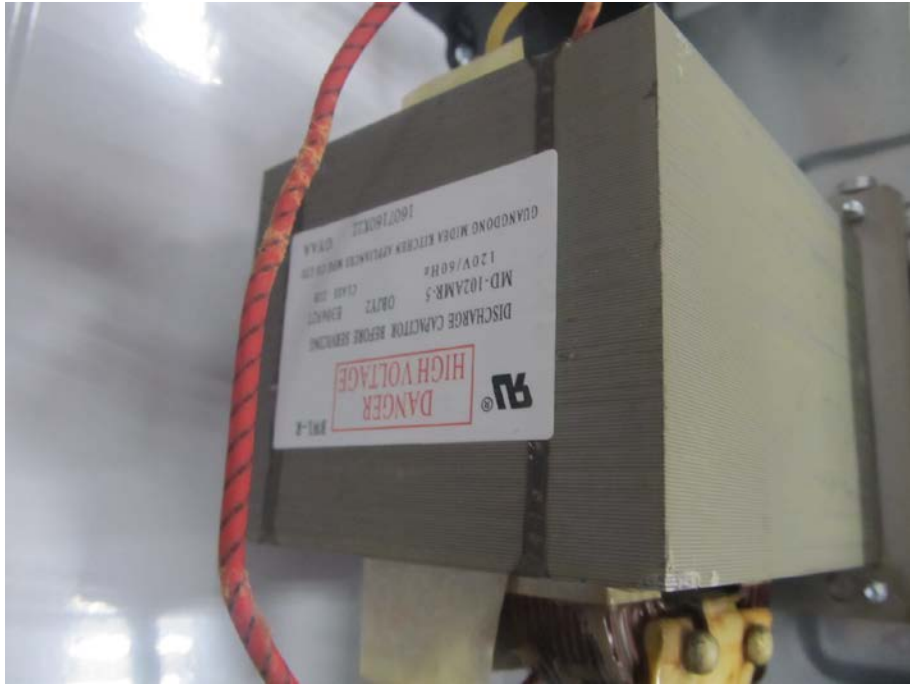
High-voltage Transformer view
