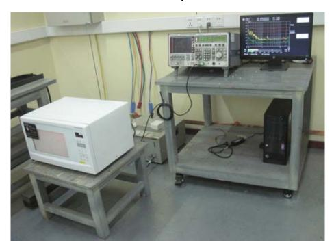
Radiated Emission Test Set-up (30 -1,000MHz):
