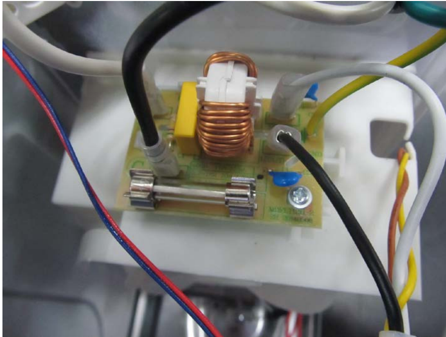
Power Filter Board Top View
