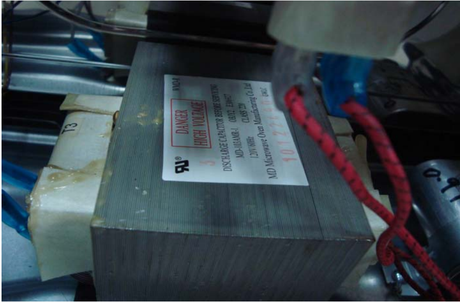
High-voltage Transformer View
