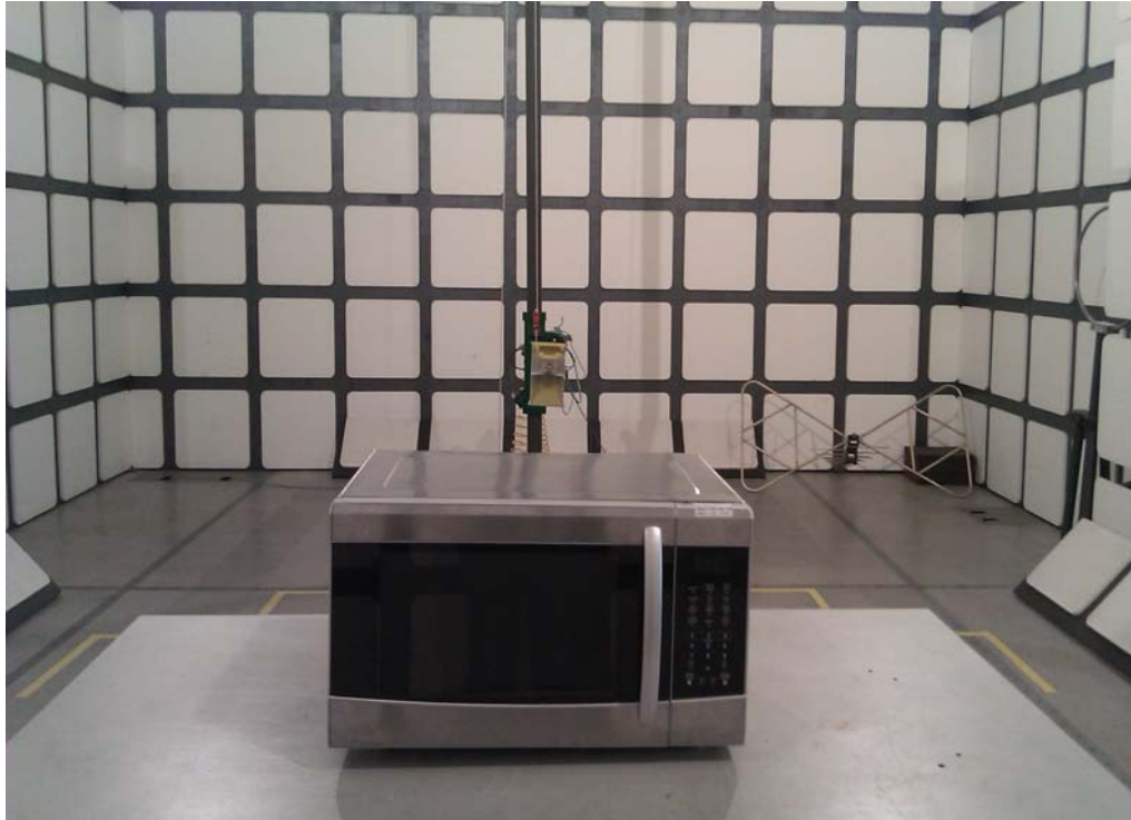
Radiated Emission Test Set-up (1~25GHz):
