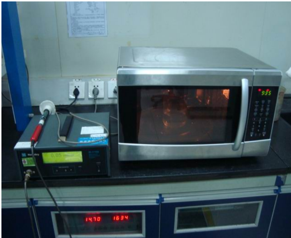
Radiation Hazard Test Set-up:
