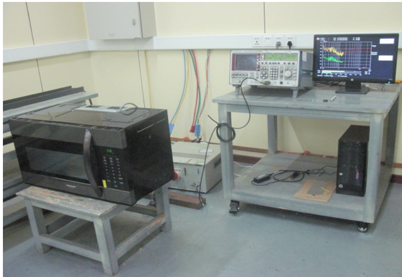
Conducted Emission Test Set-up
