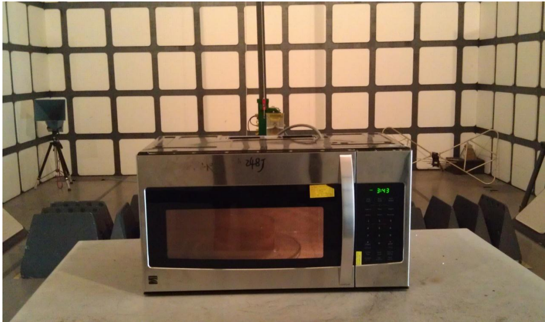
Operating Frequency Test Set-up
