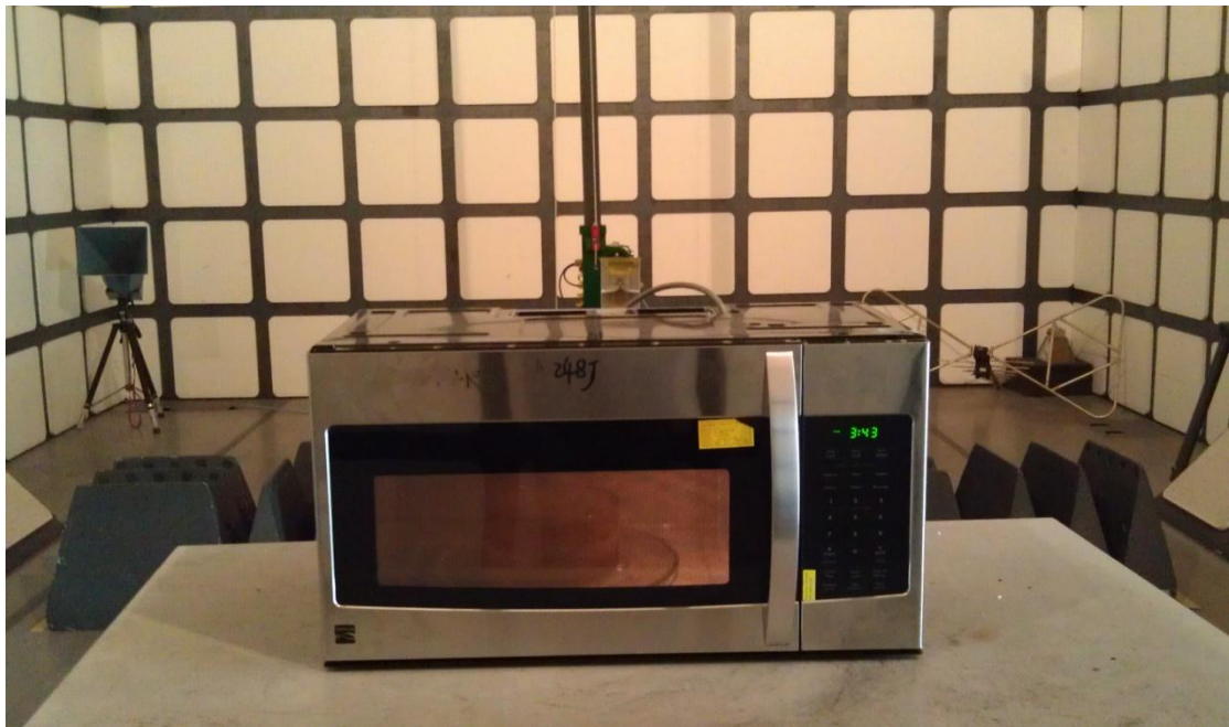
Radiated Emission Test Set-up (1-25GHz):
