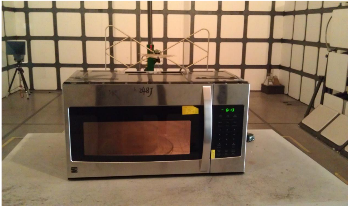
Radiated Emission Test Set-up (30 -1,000MHz)
