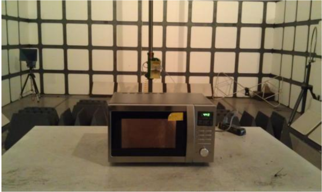
Operating Frequency Test Set-up
