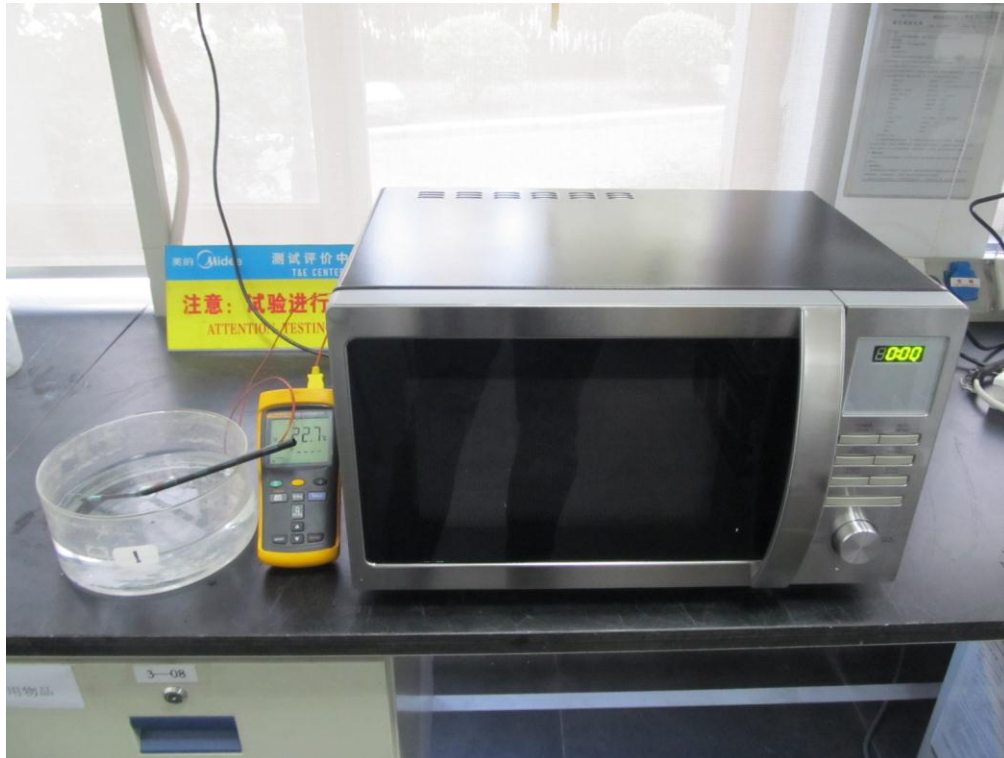
RF Output Power Test Set-Up
