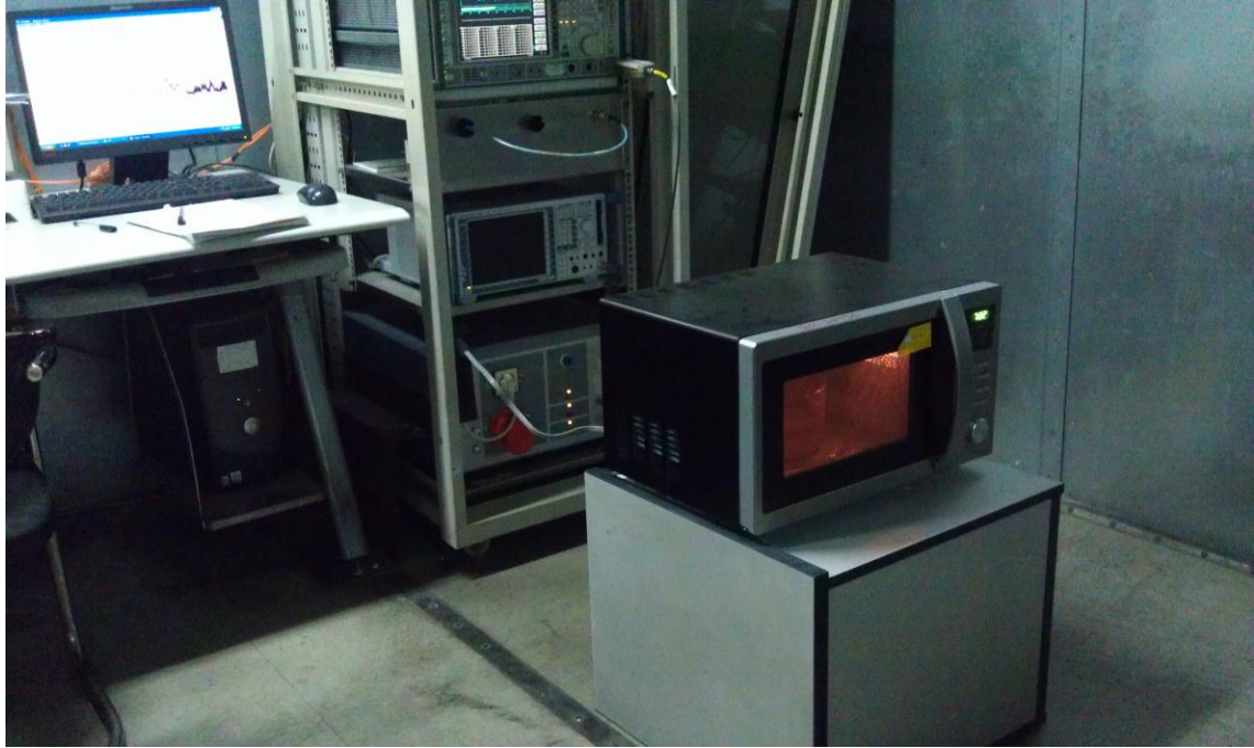
Conducted Emission Test Set-up
