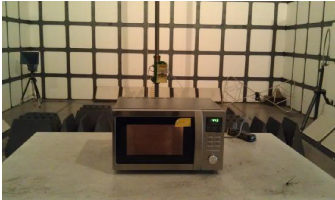
Radiated Emission Test Set-up (1-25GHz)
