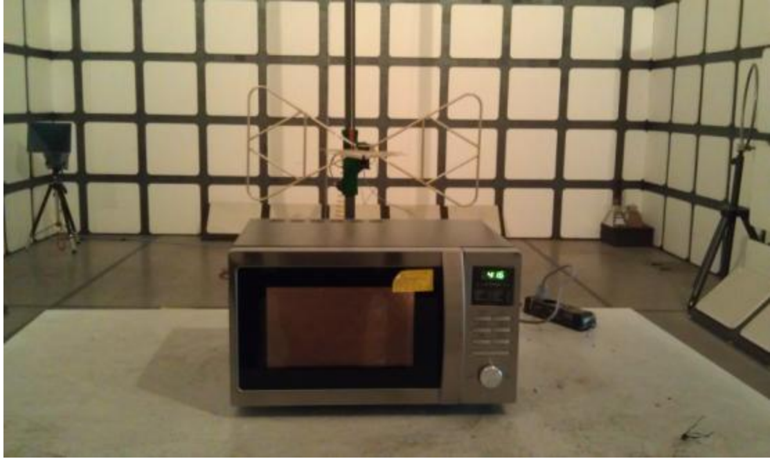
Radiated Emission Test Set-up (30 -1,000MHz)
