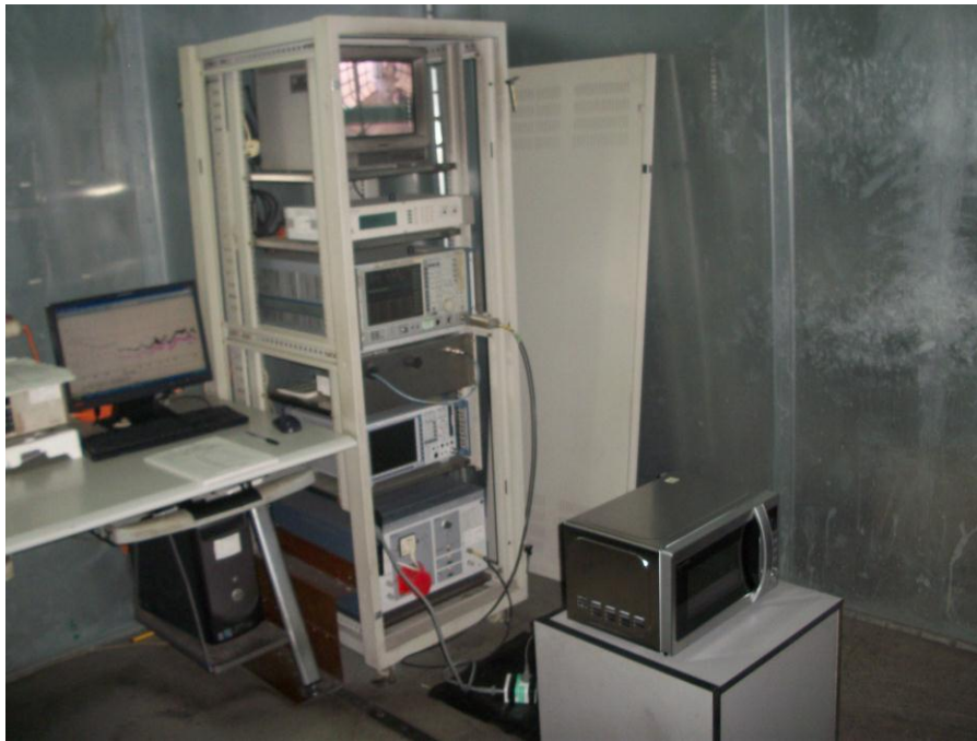
Conducted Emission Test Set-up
