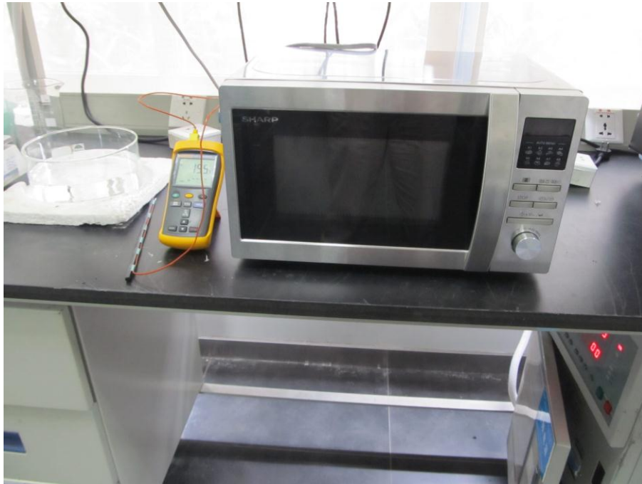
RF Output Power Test Set-Up
