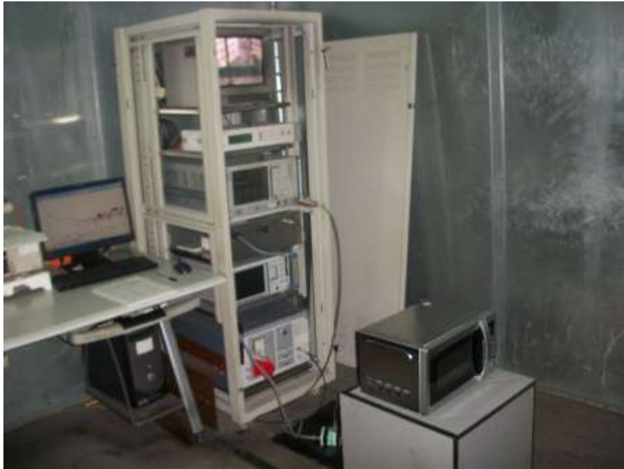
Conducted Emission Test Set-up
