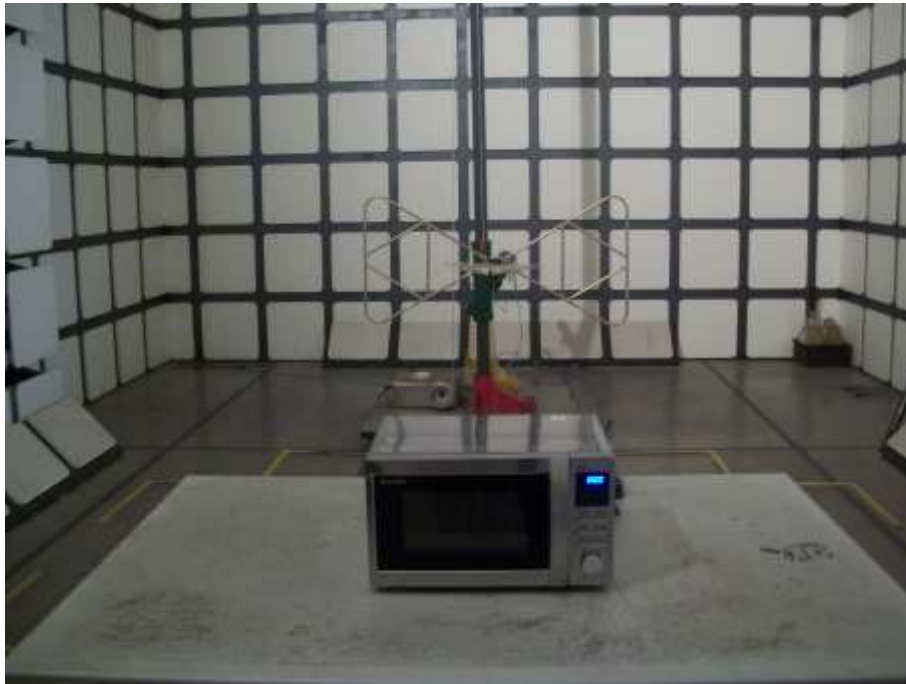
Radiated Emission Test Set-up (30 - 1,000MHz)
