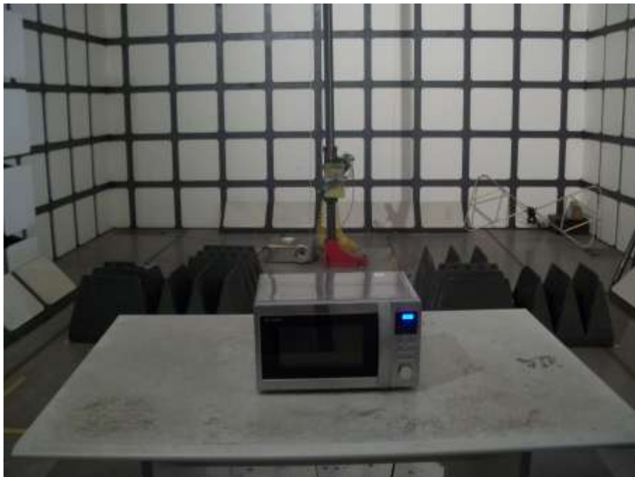
Radiated Emission Test Set-up (1-18GHz)
