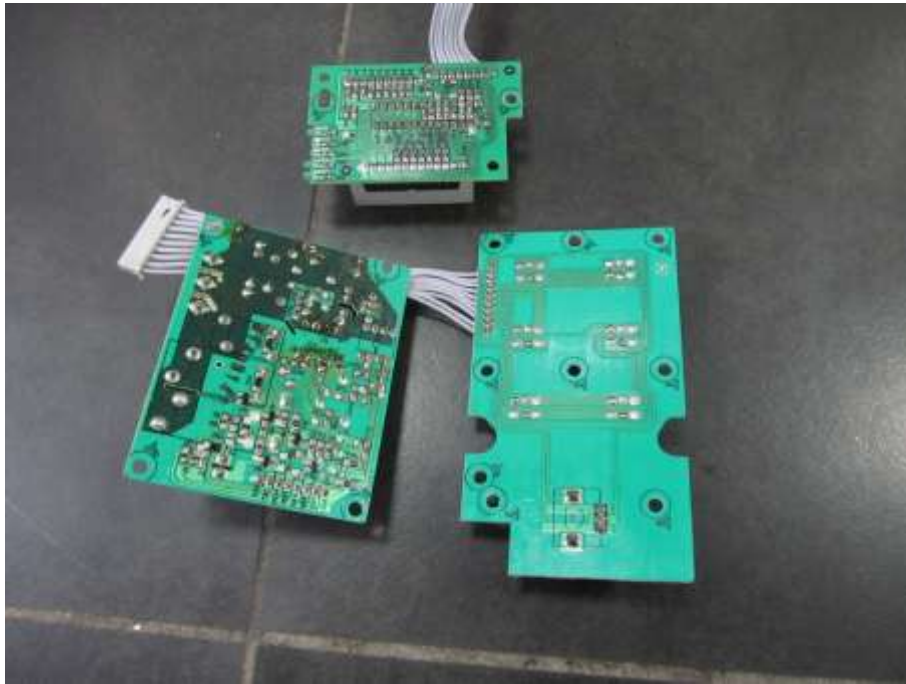
Mother board(Power board+LED display board+ Electronic Keyboard board) - Bottom View
