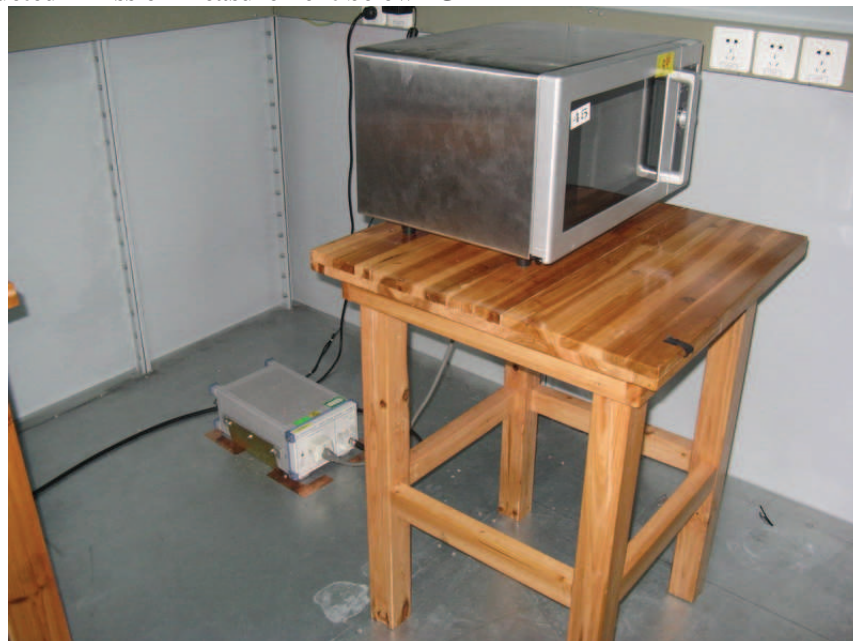
Set-up for radiation emission measurement below 1GHz
