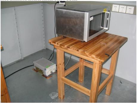
Set-up for radiation emission measurement below 1GHz
