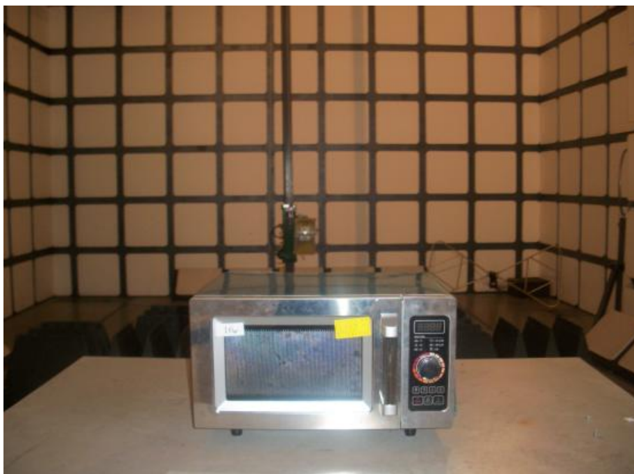
Radiated Emission Test Set-up (1–18GHz)
