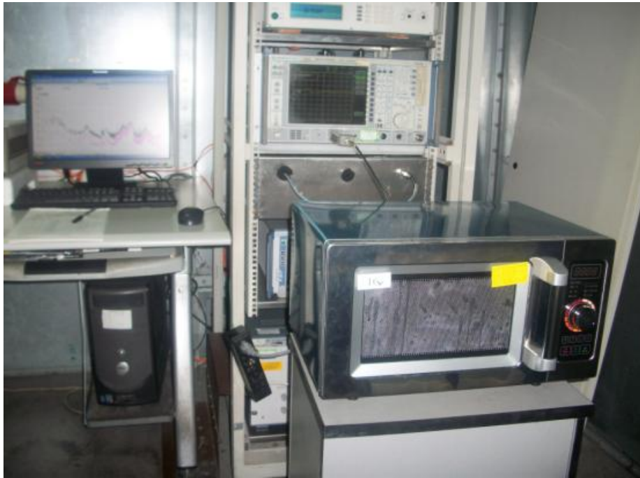
Conducted Emission Test Set-up
