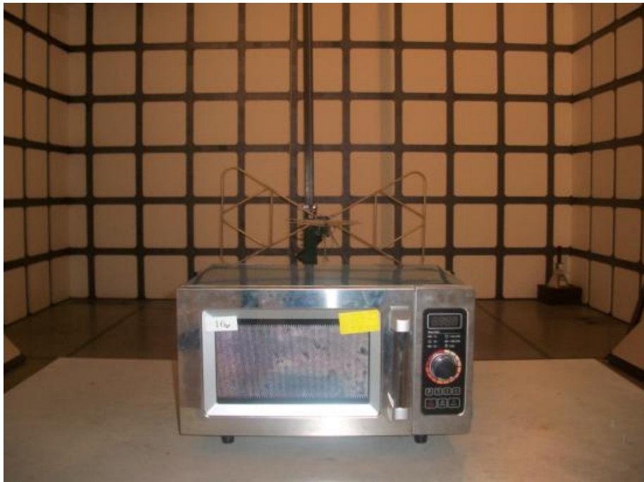
Radiated Emission Test Set-up (30 –1,000MHz)
