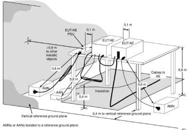
**Note:** The 0.8 m distance specified between EUT/AE/PSU and AMN/AAN, is applicable only to the EUT being measured. If the device is AE then it shall be >0.8 m.
