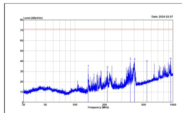
Project No. : RWAP202400177 Test Mode : Microwave Test Voltage : AC 120V/60Hz
