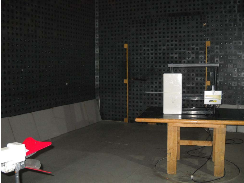
Photograph No.11 Spurious emissions measurement setup in the anechoic chamber in 1-18 GHz, EUT with flat panel antenna
