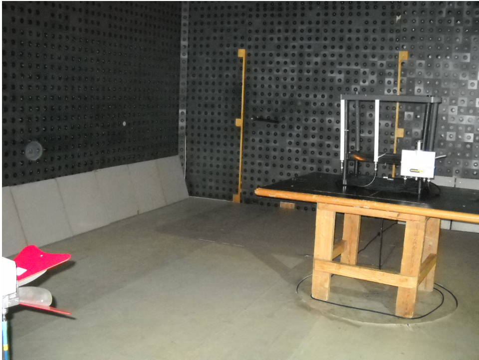
Photograph No.7 Spurious emissions measurement setup in the anechoic chamber in 1-18 GHz, EUT with omnidirectional antenna
