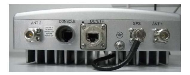
Photograph No.3 Base station WiN7258 interface panel view
