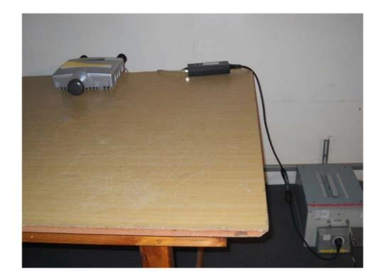
Photograph No.14 Conducted emissions measurement on AC line setup
