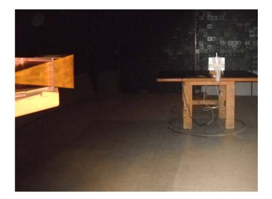
Photograph No.10 Spurious emissions measurement setup in the anechoic chamber in 26.5 -40 GHz
