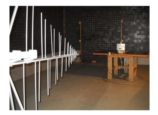
Photograph No.8 Spurious emissions measurement setup in the anechoic chamber in 1-18 GHz
