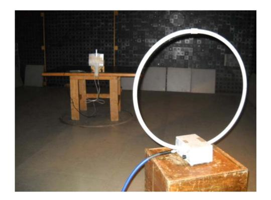
Photograph No.7 Spurious emissions measurement setup in the anechoic chamber in 30 -1000 MHz
