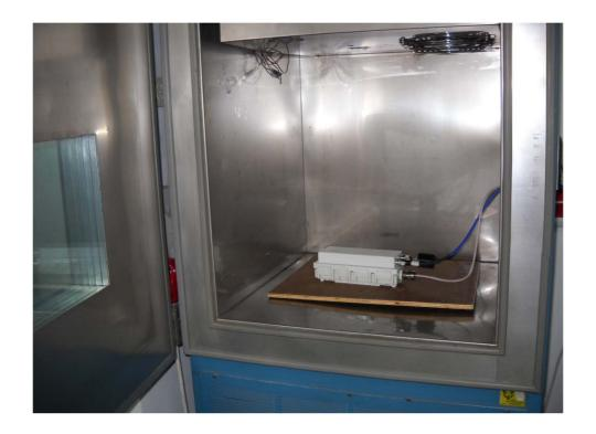
Photograph No.13 Conducted emissions measurement on AC line setup
