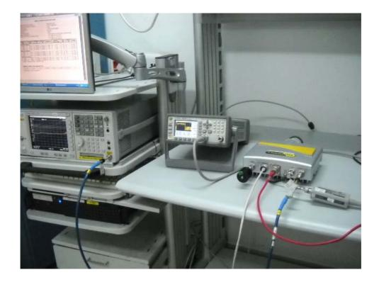
Photograph No.6 Spurious emissions measurement setup in the anechoic chamber below 30 MHz
