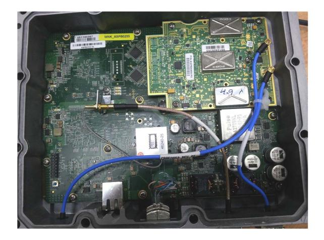
Photograph No.2 Base station WiN7249 internal view with RF module removed
