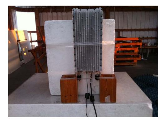
Photograph No.7 Spurious emissions measurement setup at the OATS, close view
