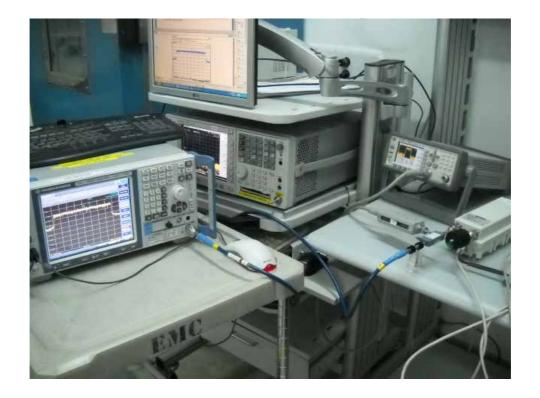
Photograph No.4 Conducted spurious emissions measurement setup
