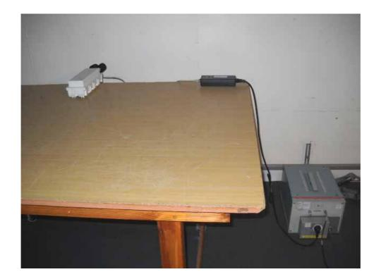
Photograph No.18 Conducted emissions measurement on AC line setup
