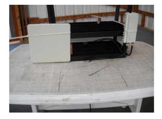
Photograph No.17 Conducted emissions measurement on AC line setup
