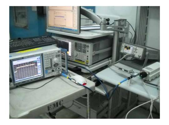
Photograph No.4 Conducted spurious emissions measurement setup
