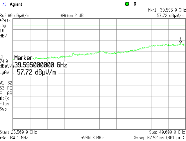
Plot 7.4.47 Radiated emission measurements from 26500 to 40000 MHz at the mid carrier frequency
