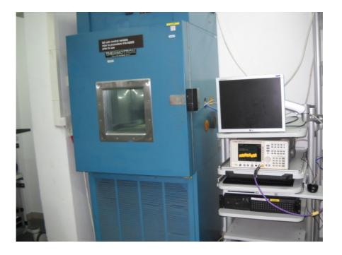
Photograph No.12 Frequency stability measurement setup
