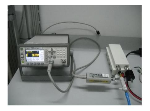
Photograph No.1 Peak output power measurement setup
