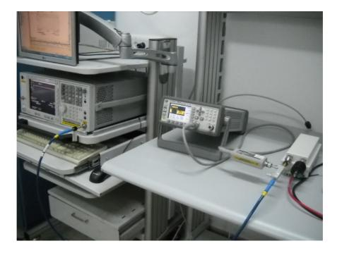
Photograph No.3 Occupied bandwidth measurement setup
