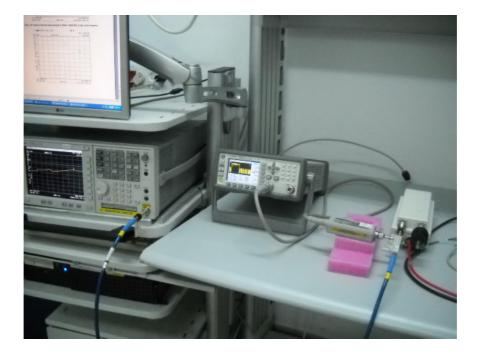
Photograph No.5 Conducted spurious emissions measurement setup
