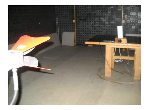
Photograph No.9 Spurious emissions measurement setup in the anechoic chamber in 18 -26.5 GHz
