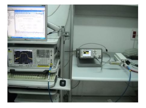
Photograph No.2 Power spectral density measurement setup
