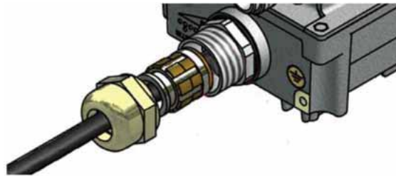
Figure 4.16. Connecting the Cable to the CPE
