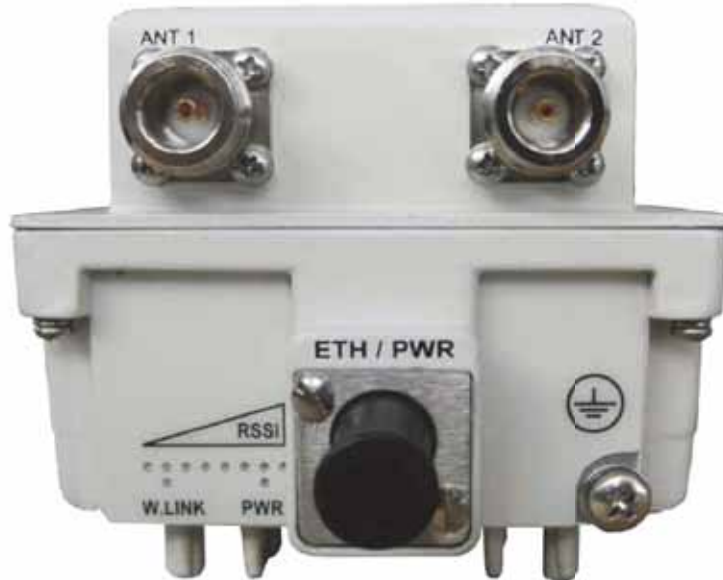
Figure 2.6. WiN5100 Connectors: AC Version
