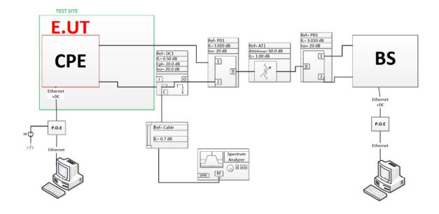
Fig. 1. The RuggedMax<sup>TM</sup> WIN5123 setup configuration.
