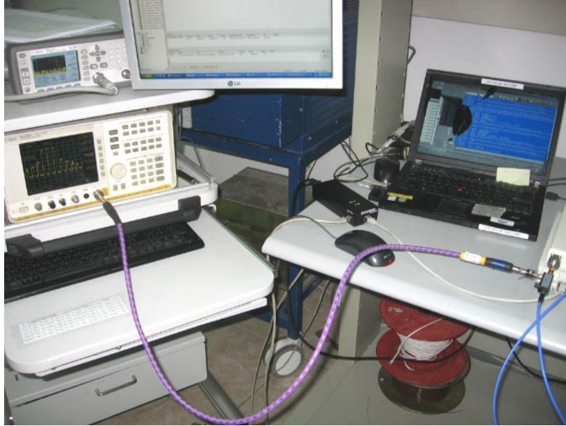
Photograph No.2 Occupied bandwidth measurement setup
