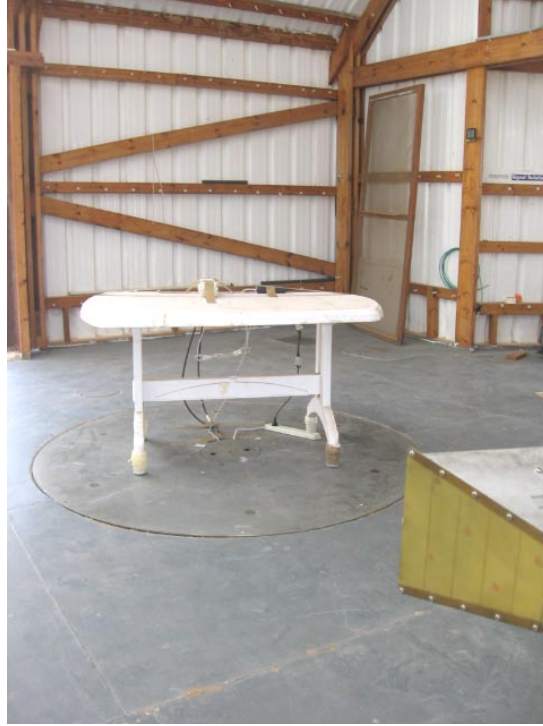
Photograph No.7 Radiated spurious emissions measurement setup at the OATS above 1000 MHz
