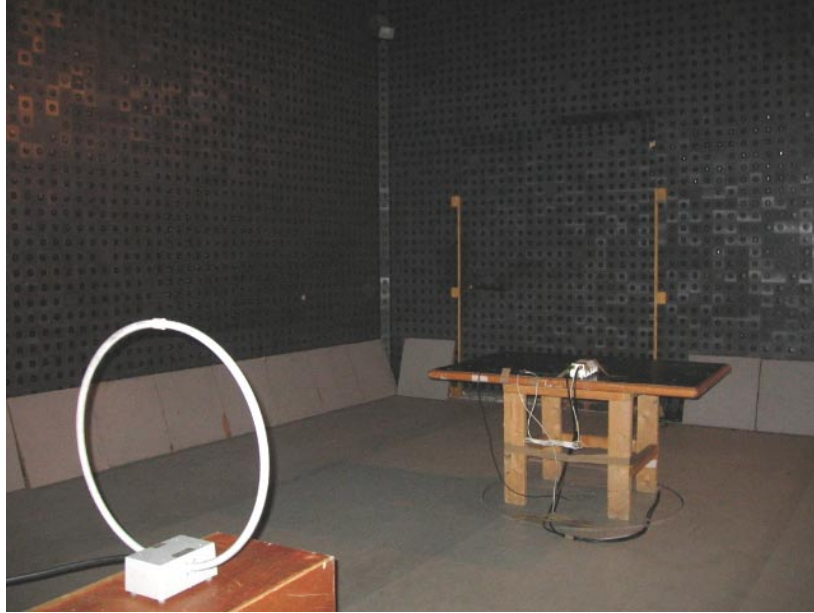
Photograph No.4 Spurious emissions measurement setup in the anechoic chamber below 30 MHz
