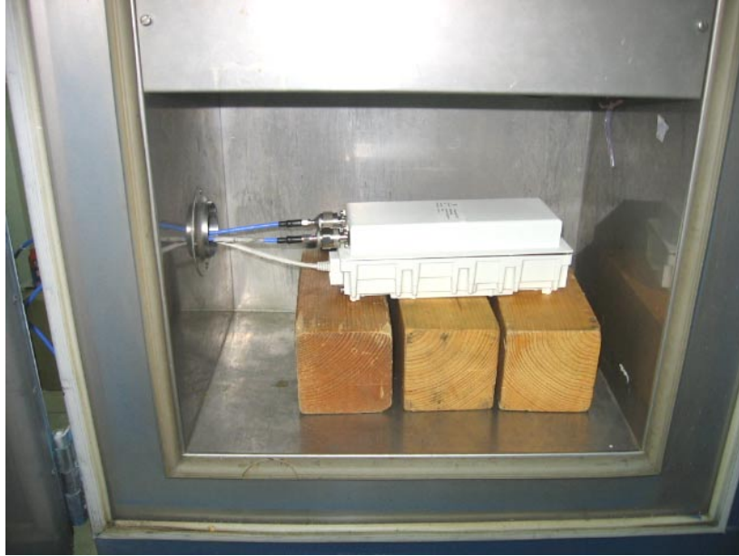
Photograph No.8 Frequency stability measurement setup
