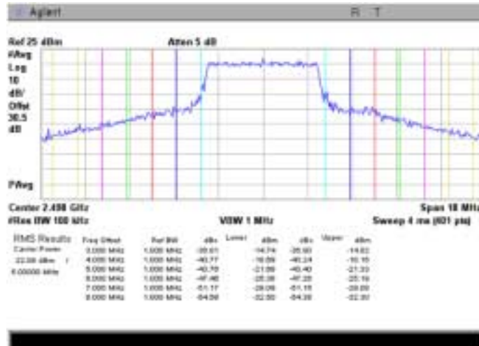
Plot 7.5.2 Emission mask test results at mid carrier frequency, 5 MHz EBW
