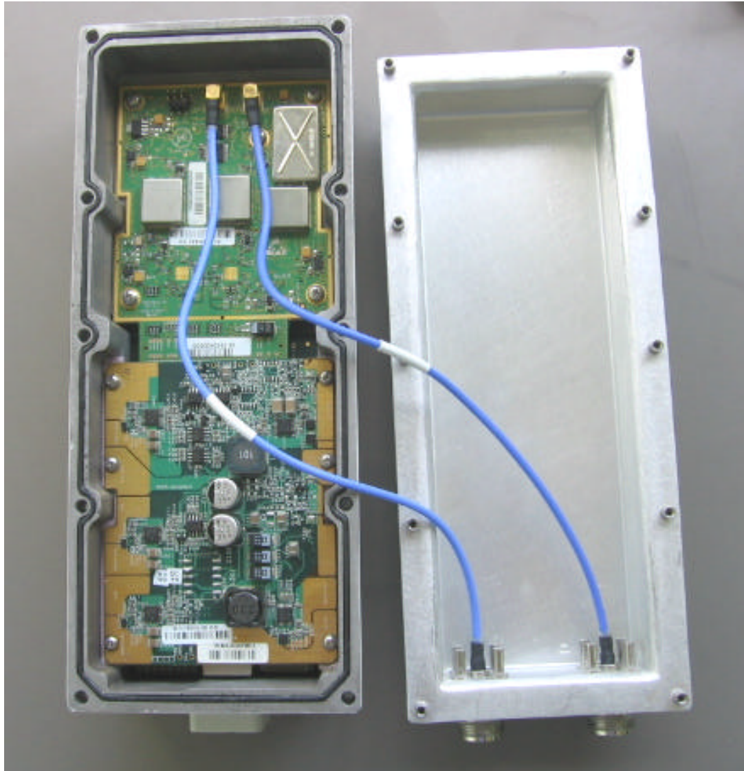
Photograph No.1 Subscriber fixed unit WiN5125-AC internal view
