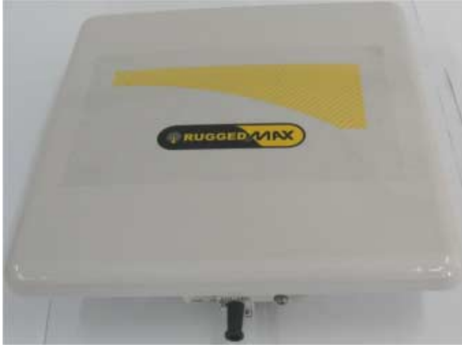
Photograph No.8 Subscriber fixed unit top view with integrated panel antenna, WiN5225
