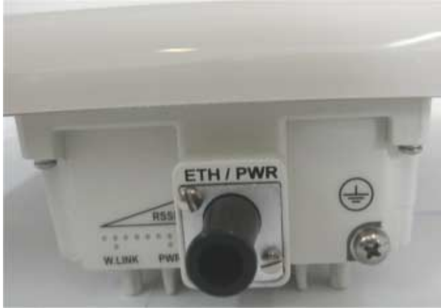
Photograph No.10 Subscriber fixed unit front view with integrated panel antenna, WIN5225
