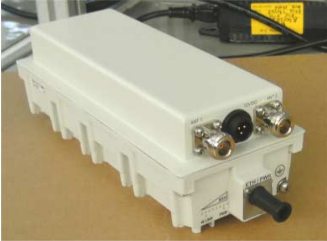
Photograph No.4 Subscriber mobile unit WiN5125-DC general view
