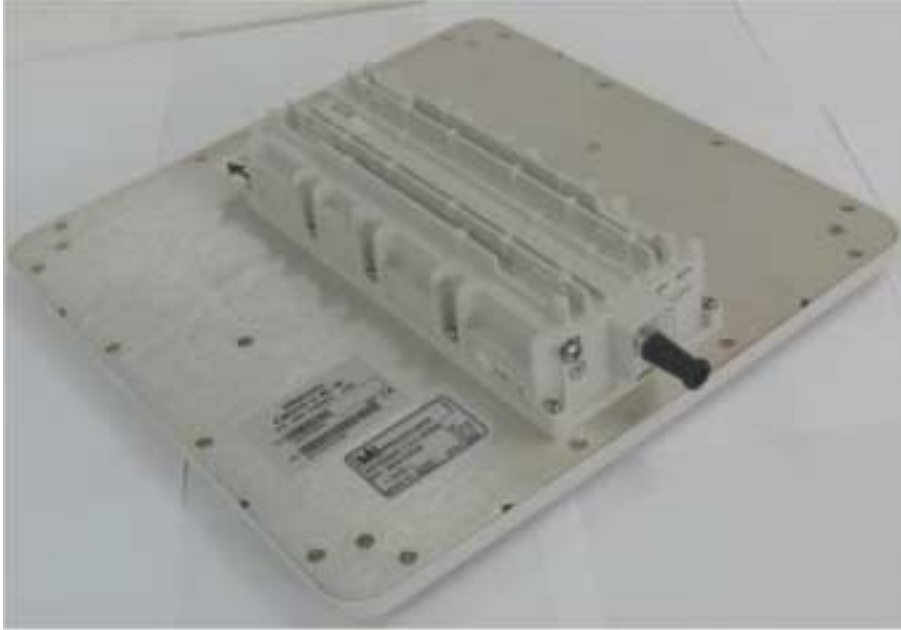
Photograph No.7 Subscriber fixed unit bottom view with integrated panel antenna, WiN5225
