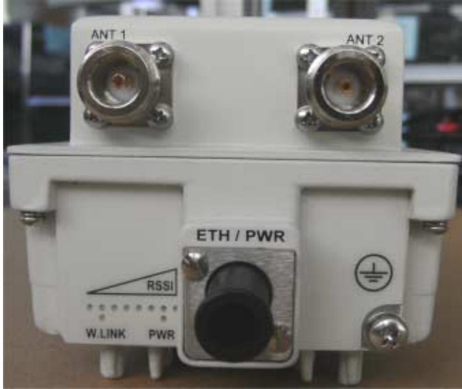
Photograph No.2 Subscriber fixed unit WiN5125-AC front view
