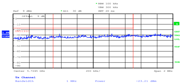
Figure 8.8-137: Lower band edge emission at 5715 MHz, channel 149, 802.11n HT20, ch1
