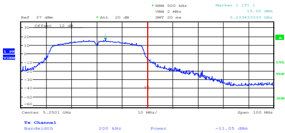
Figure 8.8-189: Upper band edge emission at 5250 MHz (ISED only), channel 48, 802.11n HT20, ch1 – reference fundamental
