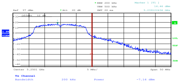
Figure 8.8-185: Upper band edge emission at 5250 MHz (ISED only), channel 46, 802.11n HT40, cho – reference fundamental
