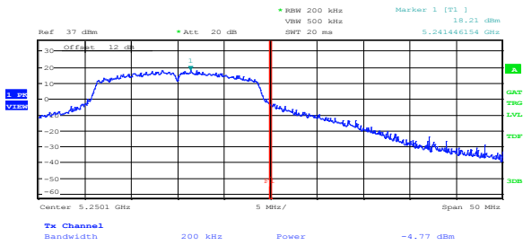
Figure 8.8-181: Upper band edge emission at 5250 MHz (ISED only), channel 48, 802.11a, cho – reference fundamental
