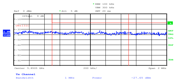
Figure 8.8-170: Upper band edge emission at 5850 MHz, channel 165, 802.11n HT20, cho
