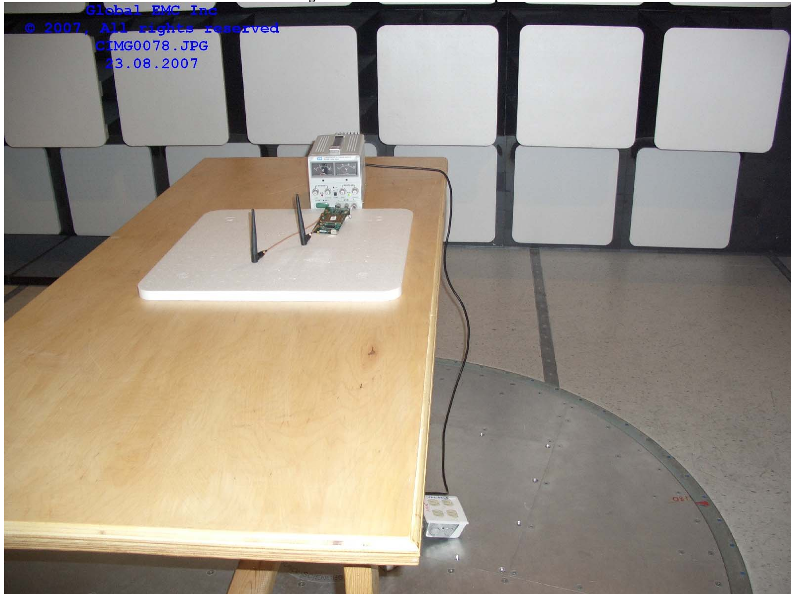
Figure 2 - Radiated Emissions Setup
