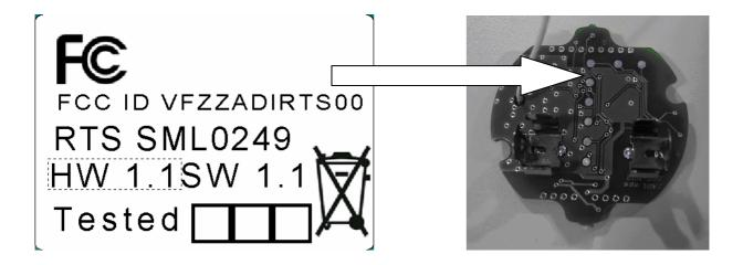
The FCC ID will be placed also outside the central receiver, in order to be visible to the end user, as show in this picture:
