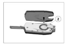
Once removed the plastic shell, pull out the battery protection cap (2).
