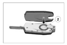
Refit protection cap (2) on the battery.
