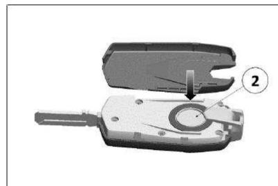
Refit protection cap (2) on the battery.
