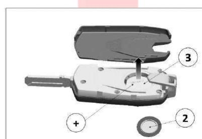
Remove the battery (3) and install a new one.
