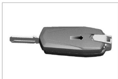
Reinstall the rear plastic shell (1) and push slightly as shown in the figures.
