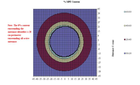
Conclusion: By inspection of percent-MPE contour plot, compliance boundary is circle, and therefore simultaneous transmission of collocated transmitter remains compliant with RF exposure.
