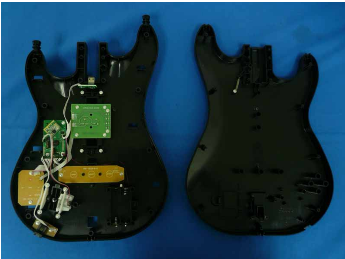
Figure 9 Inside of the EUT
