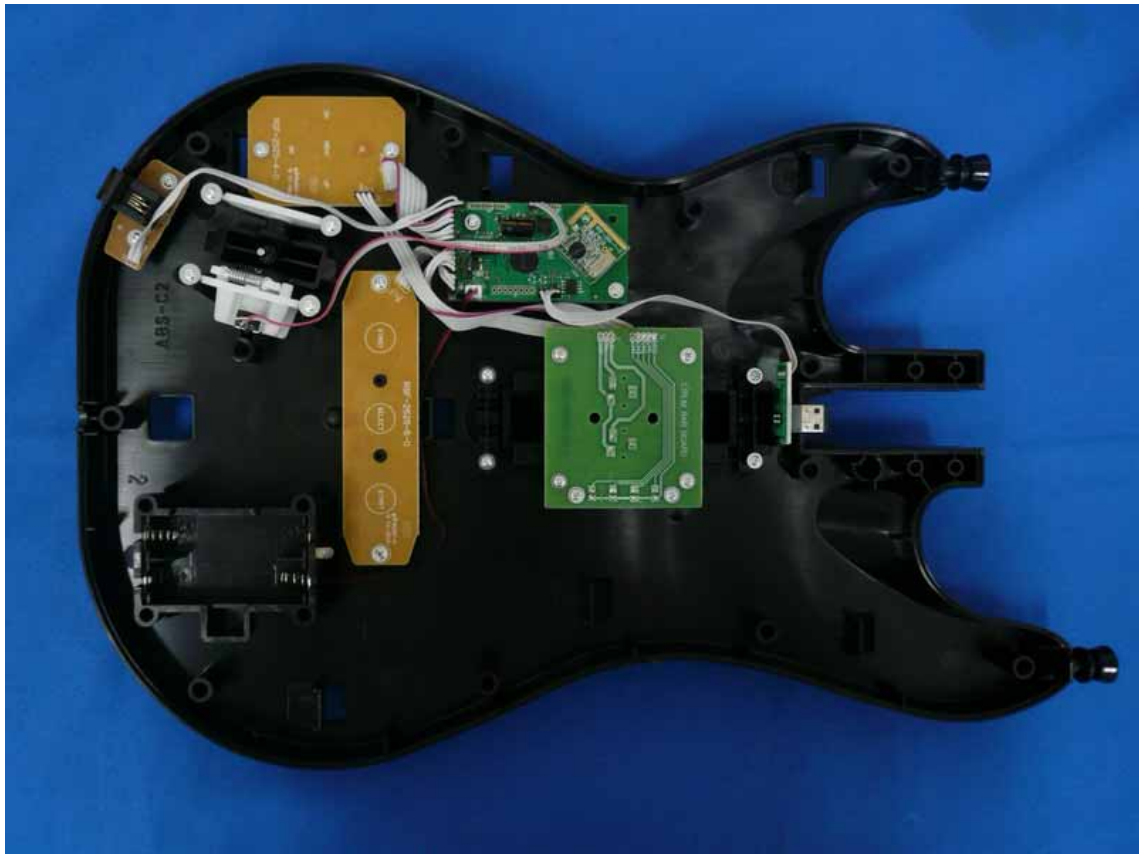
Figure 11 Components Side of the PCB
