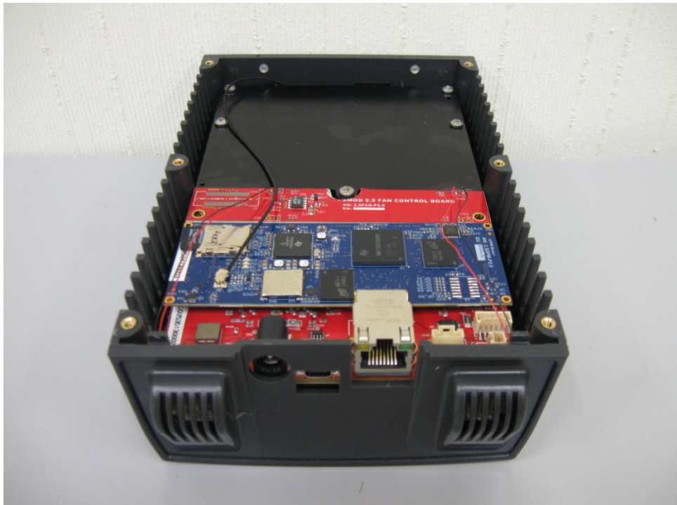
Fig-18. xModem Assembly inside Top Housing. Top View
