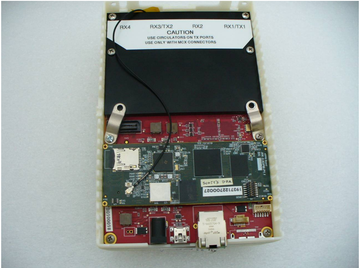
Figure 9: Internal View Showing Module Location and Clamps
