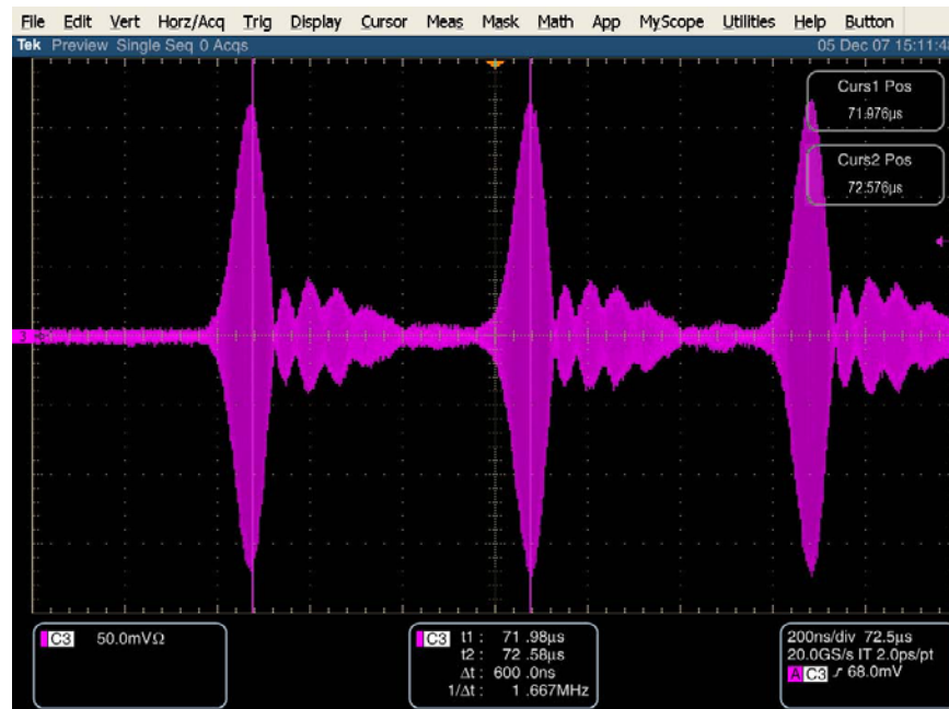
Figure 1: XG-VOIP-BTS pulse repetition frequency
