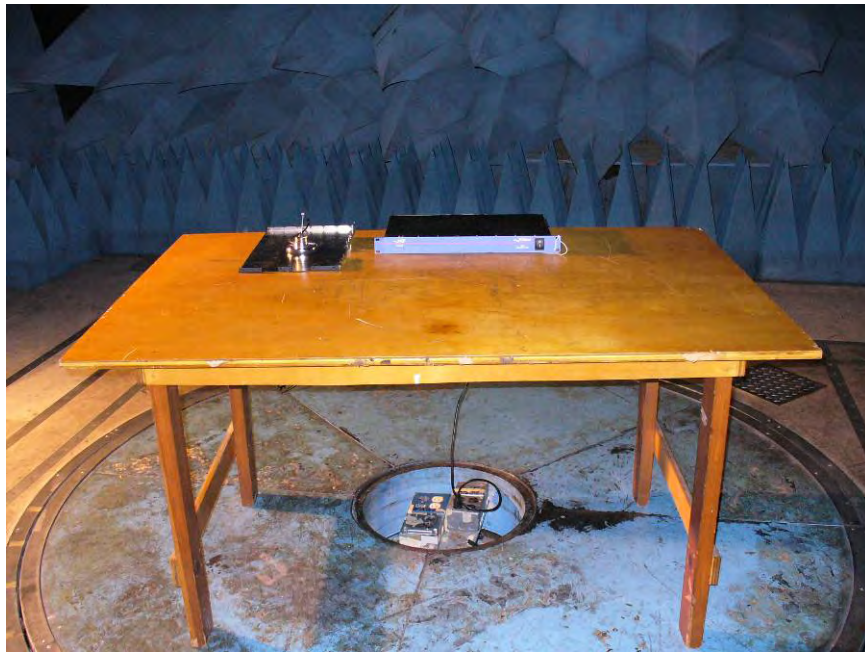
Photographs 3 & 4: Radiated Emission Setup
