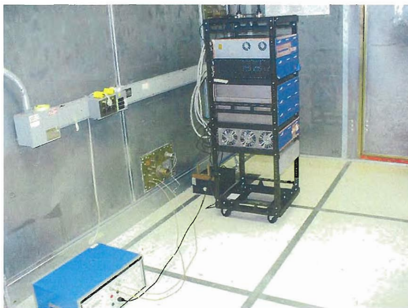
Photographs 1 & 2: Conducted Emission Setup
