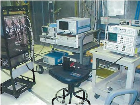
Photographs 5 and 6: Power, bandwidth and PSD Measurement Setup
