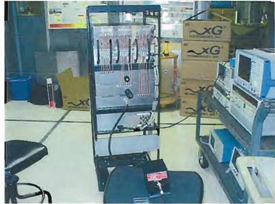
Photographs 5 and 6: Power, bandwidth and PSD Measurement Setup
