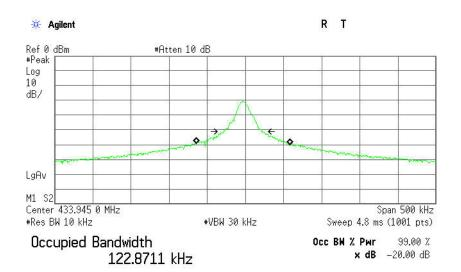
Transmit Freq Error -2.824 kHz x dB Bandwidth -2.824 kHz 50.250 kHz
